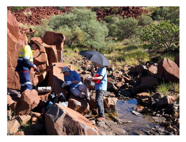
Figure 35: ASD FieldSpecPro and Konica Minolta CM-700dspectrophotometer operating on petroglyphs in the Burrup Peninsula (2013)
