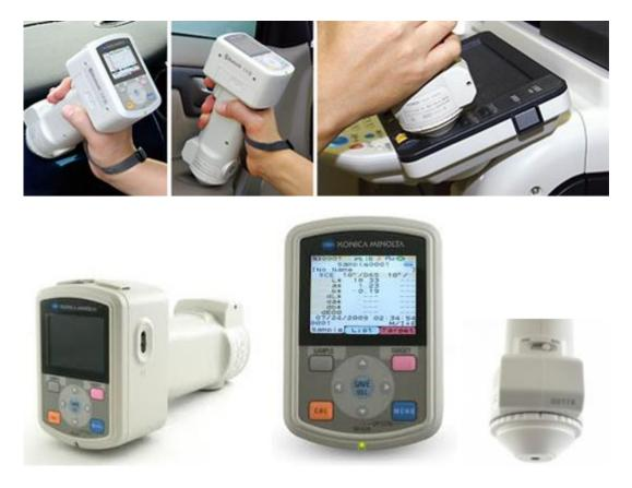
Figure 5: Konica Minolta CM-700d spectrophotometer.
